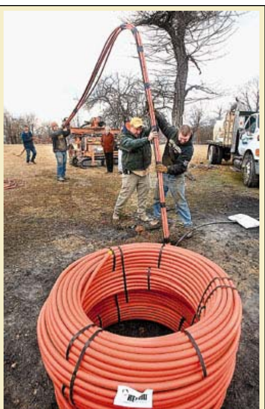
Workers feed tubing into a 300-foot hole on Thursday to measure the ground temperature at the site of the Shenandoah Valley Discovery Museum's future home in Jim Barnett Park in Winchester. (Scott Mason)
